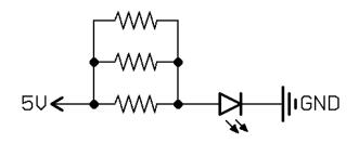
Connecting parts side-by-side. Adding resistors in parallel lowers the total resistance by making more pathways for the current to flow through. This causes the LED to become brighter.
